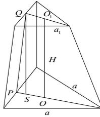
$$V = \frac{H}{3}(B_1 + \sqrt{B_1 B_2} + B_2)$$
